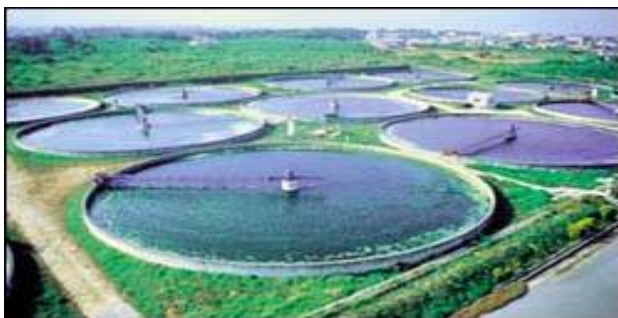
A farm in Southern Japan grows chlorella in circular pond and New Ambadi farm in India grows spirulina in raceway style ponds.
